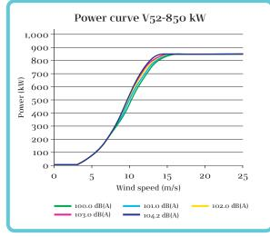
The figure above illustrates the power curves at different sound levels for the V52-850-kW turbine, which is equipped with OptiSpeed®.
