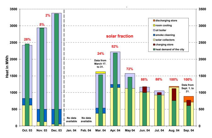
Fig. 2.18: System heat balance from October 2003 to September 2004 according to heat meter data
