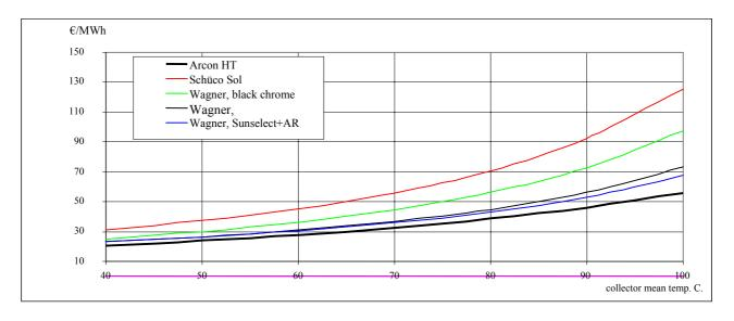
Fig. 2.7. Heat production prices from different roof modules.
