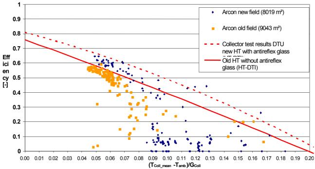
Collector field efficiency Arcon collector fields.
