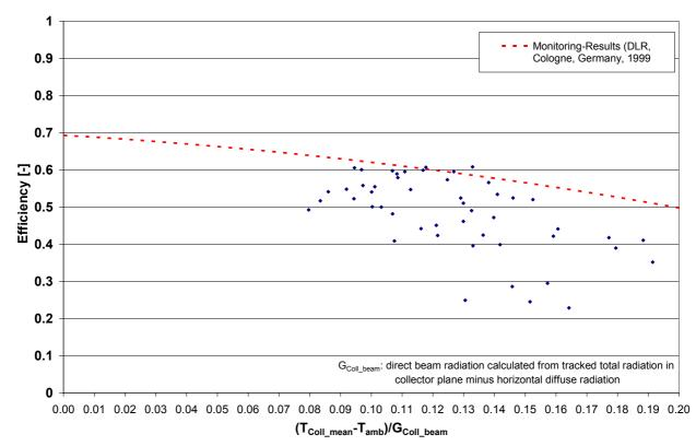
Fig. 2.27: Collector field efficiency IST field (parabolic troughs, 211 m<sup>2</sup>)
