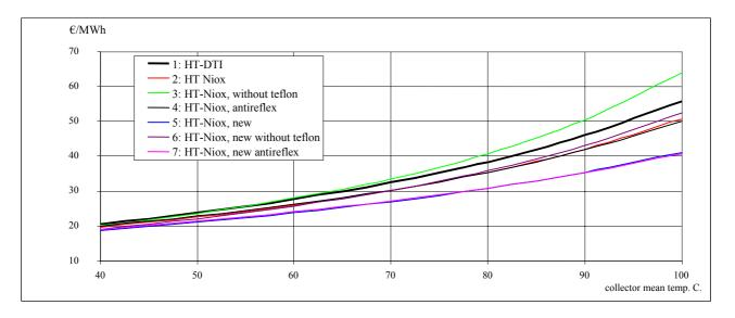
Fig. 2.3. Production price for heat for different collector combinations with Sunstrip absorbers.
