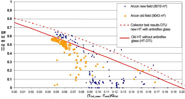
Fig. 2.23: Collector field efficiency Arcon collector fields
