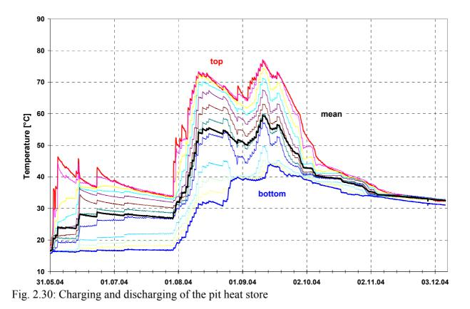
The ground around the pit heat store is heated up due to the transmission heat losses through the side walls and the bottom. The yearly mean temperature of the surrounding ground will increase in the first years because of these heat losses. After a start-up period of three to five years, where the yearly heat losses will continuously decrease, the yearly mean ground temperatures will not change anymore and the store is operating under steady-state conditions.
