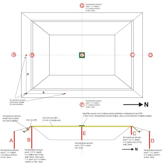
Fig. 2.17: Monitoring sensors in and around the 10 000 m<sup>3</sup> seasonal pit heat store
