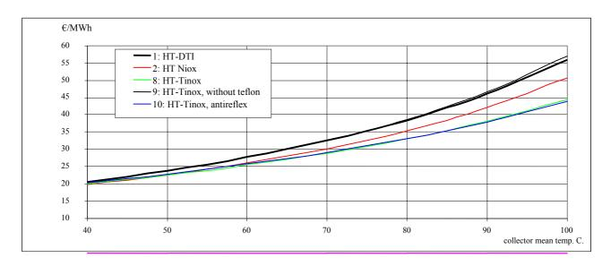
Fig. 2.4. Production price for heat for different collector combinations with Tinox absorbers.
