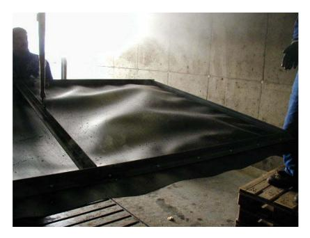
Fig. 2.8. Expansion experiment. 2.5 mm HDPE. 70 °C.
