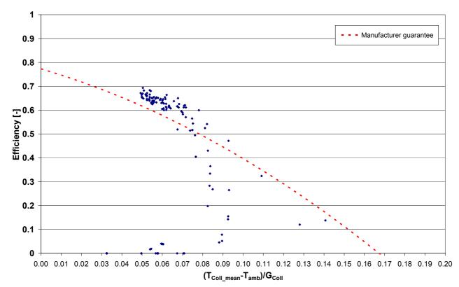
Fig, 2.24: Collector field efficiency GJ field (881 m<sup>2</sup>)
