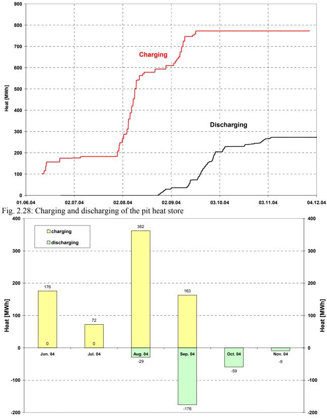
Fig. 2.29: Heat balance of the pit heat store from March to November 2004
