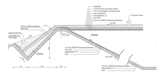
Fig. 2.10. Cross section of the edge of the pit storage.
