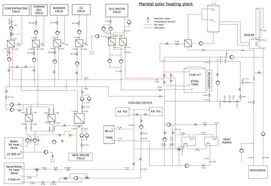
Fig. 2.16: Hydraulic plan of the Marstal solar heating plant with monitoring sensor positions
