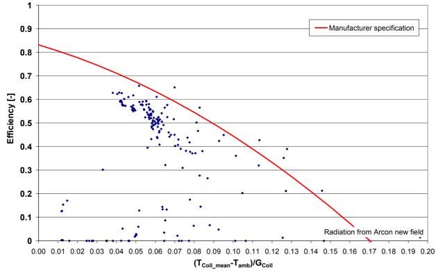
Fig. 2.25: Collector field efficiency Wagner field (103 m<sup>2</sup>)
