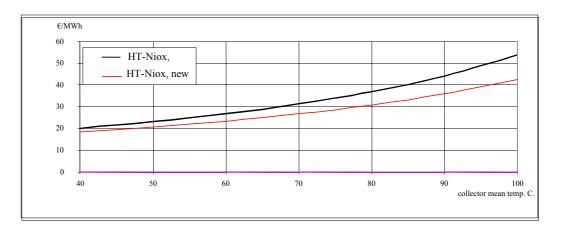
Fig. 2.6. Production prices ( $\in$ /MWh) for the older and the new ARCON-HT collector
